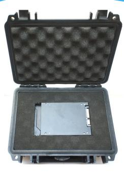
Original observation flight data is recorded on removable medium. In addition, the algorithm of the original data recording on removable medium includes recording of non-displaced reduced (preview) images, which are simultaneously displayed on the operator's monitor during an observation flight.
