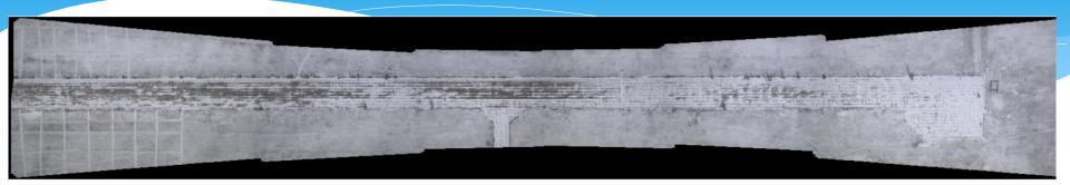
Example of an Open Skies digital imagery product from low altitude channel, consisting of six sub-frames.
