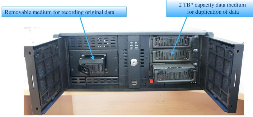
\* - Processing server has the capability for simultaneous recording of observation flight data in OSDDEF format on five data media (three internal and two external USB 3.0 data storage-devices) with an average speed approximately 60 MB/sec for each data medium.
